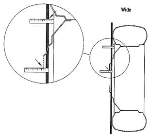
To Measure Inside Wide Setting Wheels If the center is set out past the edge of the tire, measure from the straight edge to the outside face of the center. Next, measure from the straight edge to the rim's edge. Add this amount to the previous measurement to obtain the inside wheel measurement.
