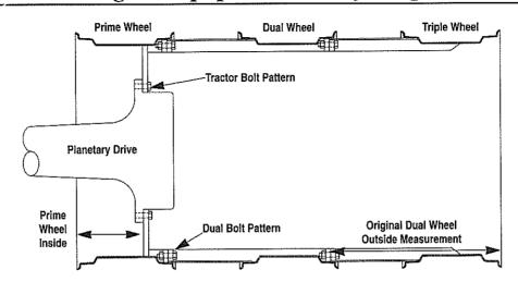
This system use the original prime as the prime wheel. A new dual wheel consists of a plate center, a spacer band with a center, and gussets welded into the rim. This dual wheel will bolt to the dual bolt pattern on the tractor. The original dual wheel becomes the triple by bolting to the plate center in the new dual wheel.
