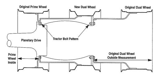
This system uses the original prime wheel as the prime wheel. A new dual wheel consists of a plate center, a spacer band with a center, and gussets welded into the rim. This dual wheel bolts to the main bolt pattern on the tractor. The original dual wheel is used as the triple by bolting to the plate center in the new dual wheel.
