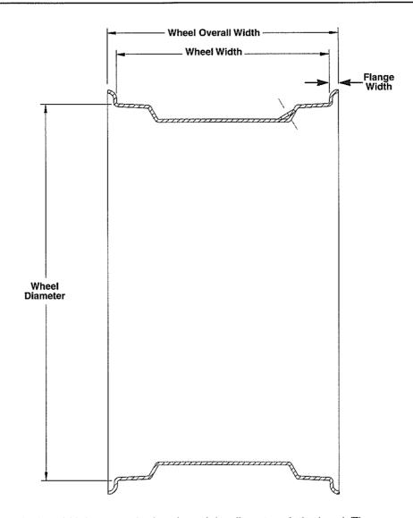
The wheel size given is the width between the beads and the diameter of the bead. The measurements used in this catalog are from the outside edge of the wheel. This is the best way to obtain measurements from a wheel with a mounted tire. Because of the process in which the wheel is made, the flange width can vary. This will cause the wheel outside measurement to vary.
