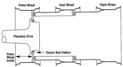
This system is a complete kit consisting of twelve wheels. Kit is used when changing tire size or replacing a current dual system to the heavy duty Tiger Cat-style triple system.
