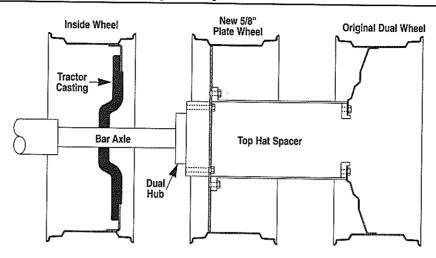
This system uses the original 10-bolt dual hub. The dual wheel is removed and a 5/8" plate wheel bolts to the dual hub. A top hat spacer bolts to the new plate centered wheel and the original dual wheel bolts to the top hat spacer for the triple wheel.
