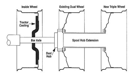
This system uses the original 10-bolt dual hub and dual wheel. Eight of the 10 bolts are removed. The spool hub extension bolts to the dual wheel and hub with eight longer bolts (furnished.) The triple wheel bolts to the hub extension.
