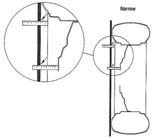
To Measure Inside for Narrow Setting Wheels If the center is set even with or in from the edge of the rim. repeat the above procedure on the inside of the wheel. This will give you the inside wheel measurement.
