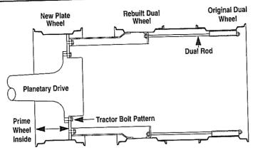
This system uses a new plate centered prime wheel. The original prime wheel is rebuilt by welding a spacer band consisting of a center, and gussets into the original prime wheel to be used as the dual wheel. The existing center hole is cut bigger for easier access to the prime wheel bolt pattern. (Original prime wheel may be rebuilt or exchanged.) The dual wheel, spacer band, and rods are utilized as the triple wheel.
