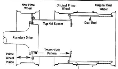
This system uses a new plate centered prime wheel. A top hat style spacer bolts to the new prime wheel with a separate bolt pattern and the original prime wheel bolts to the spacer and become the dual. The original dual wheel, spacer band, and rods become the triple.
